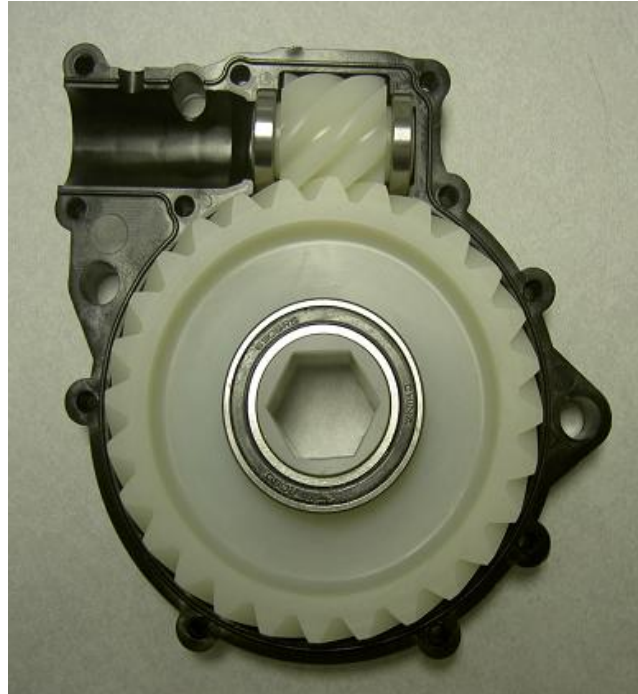
Fig. 19 Crossed helical gearbox
