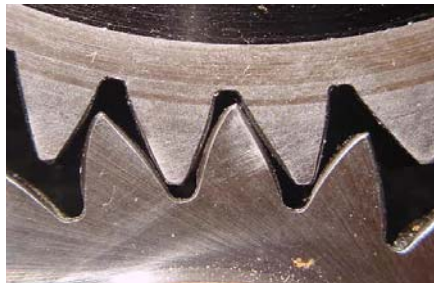
Fig.11 Gears with asymmetric teeth
