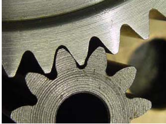
Fig.10 Gears with optimized fillets
